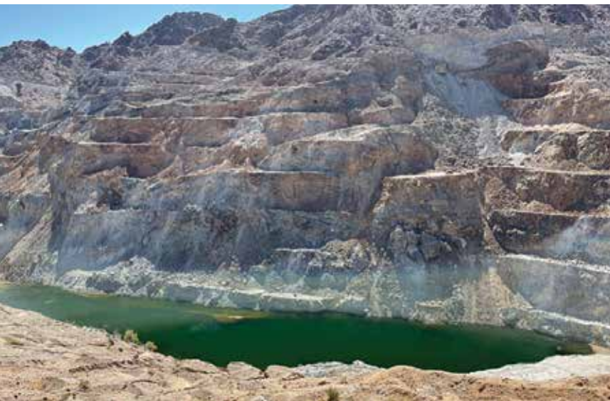
Pit lake from an abandoned gold mine, Imperial County, CA. Pit lakes often have poor water quality and can be extremely acidic, requiring perpetual treatment. All photos this spread by Jared Naimark.
