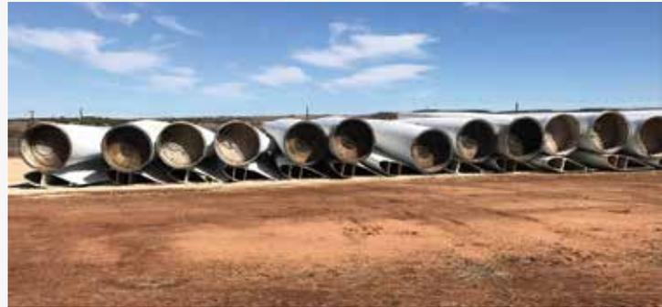
***These wind turbine blades are stored until they can (perhaps) be recycled. These blades are 121 feet long, weigh 8 tons, and are cut up into 50 sections. The round parts are where the blade attaches to the hub. Photo by Don Lilly, Global Fiberglass Solutions***
