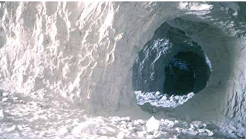
**Chalk white volcanic ash (pumicite) interior of the Old Dutch Cleanser mine workings - room and pillar mining. Photo by Mark Faull**
